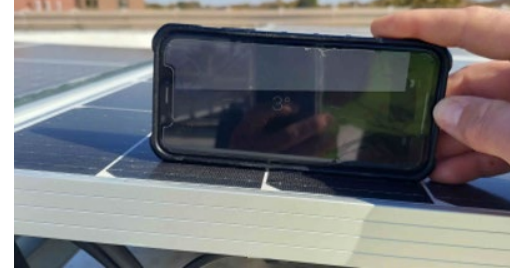
Tilt Angle: Photo showing the angle utilized for applicable flat roof projects. This angle should be consistent with all submitted project design documentation.
